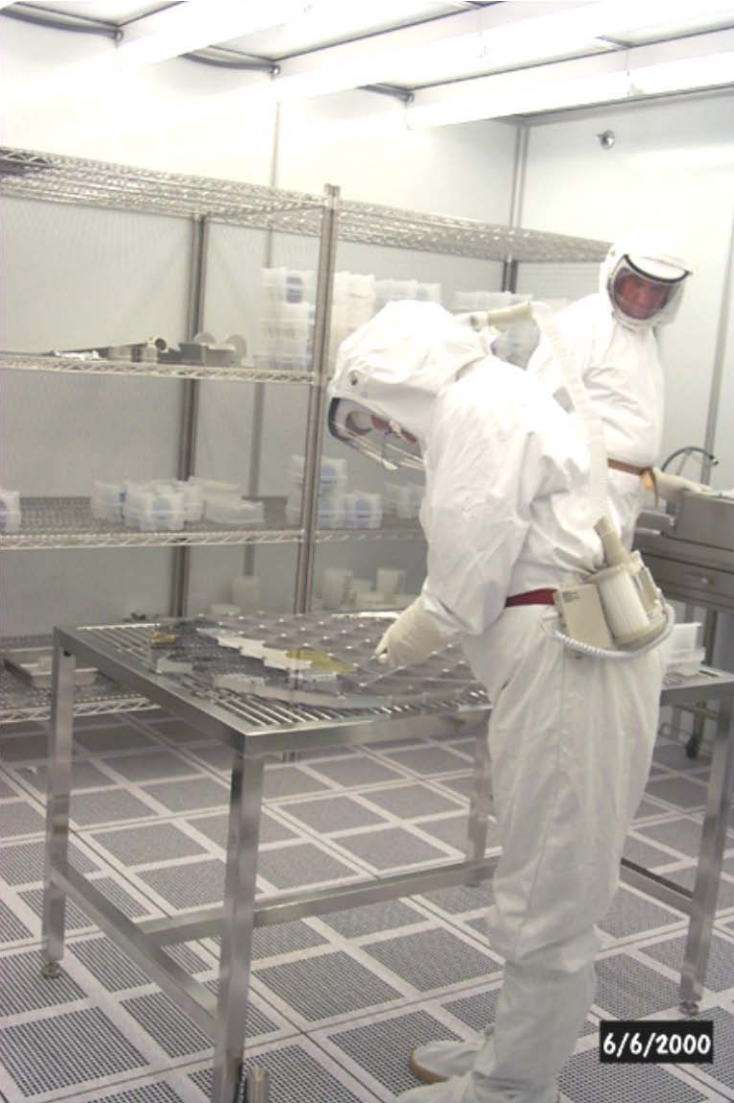
Fig. 5-4. Dryden suit completely envelops person. Self-contained battery motor forces exhaled breath through HEPA filters.
