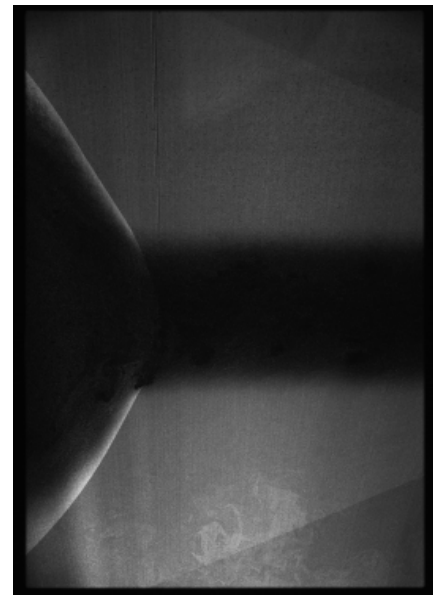
Figure 4: Raw PIV image illustrating flow seeding at the measurement plane in the tunnel. Canopy bow shock and capsule wake shock are readily observed.
