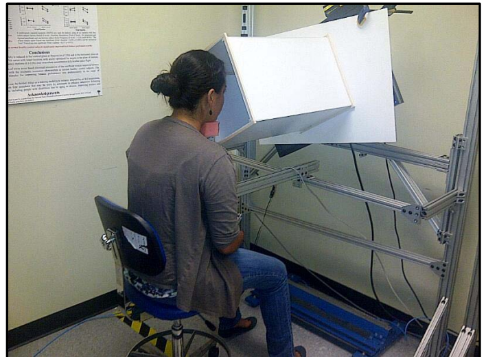
Figure4. Rod and Frame Test Apparatus. Demonstration of maintaining an upright position in the chair with chin resting on a foam cube in front of the frame and operating remote control.
