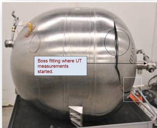
A-Tanks P0251 P0092 failed at Elliptic end
