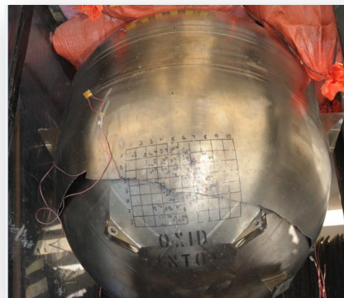
B-Tank with crack shown in the impacted area
