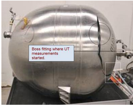
Figure 2. Tank #0251 failure at Ellipsoidal end. Tank #0092 exhibited the same failure.
