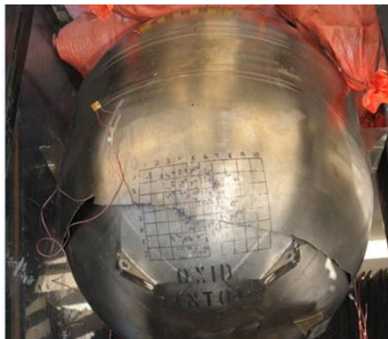
Figure 3. Tank #0062 failure at the damaged area.
