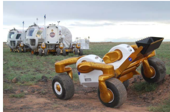
Figure 2. Centaur 2 with Glenn Research Center Bucket and Space Exploration Vehicles in background.
