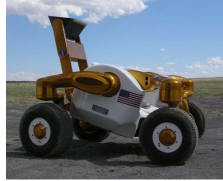
Figure 8. Glenn Research Center Bucket. Mounting to C2’s aft face was inspired by the GRC Bucket. 7
