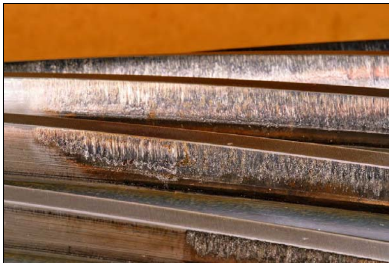
Figure 3. High-speed shaft gear set damage
