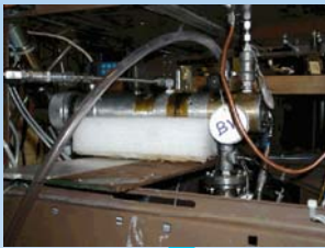
GaTech high-response fuel valve in characterization rig in CE7A
