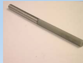
Modified MEMS-DCA package to support 800°C pressure sensor operation.
