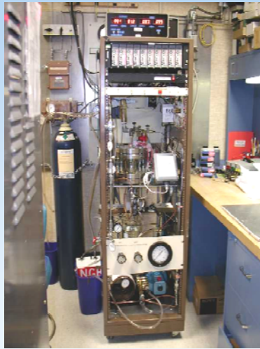
Valve, Feed-system Characterization Rig at NASA GRC
