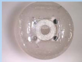
Newly developed 800°C sealing glass demonstrated on a dummy sensor and AIN package header.
