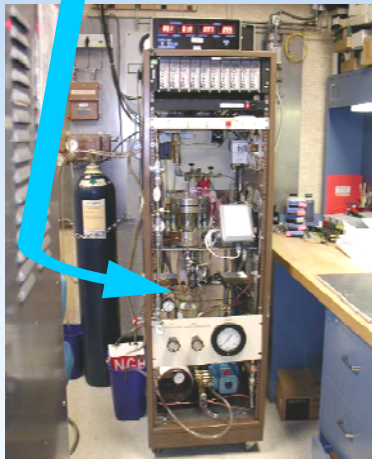
GaTech high-response fuel valve in characterization rig in CE7A
