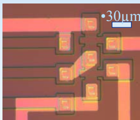
Differential amplifier circuit using two SiC transistors.
