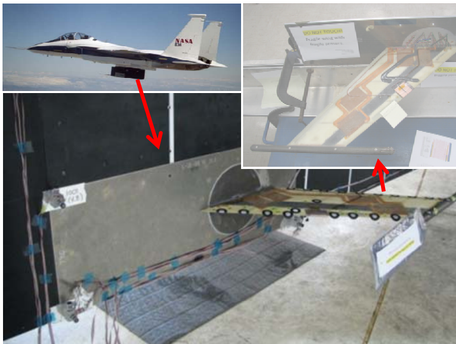
Figure 2: Aerostructures Test Wing 2 mounted on F15B pylon for the flight testing.
