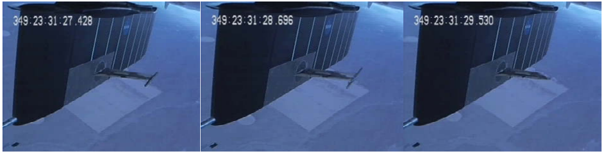
Figure 9: Classical bending and torsion flutter during flight test
