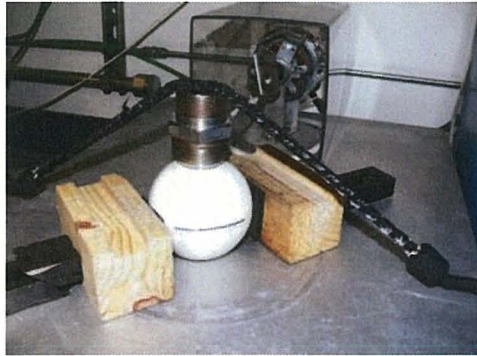
Figure 13. showing Spherical vessel Testing using 27 Hz cyclic input
