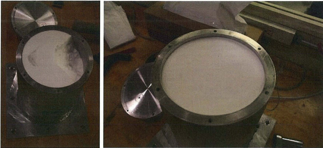
Figure 3. : Glass Bubbles after X-axis vibration, 4% void (left) and after Z-axis vibration, 2.5% void (right). Photographs of typical results
