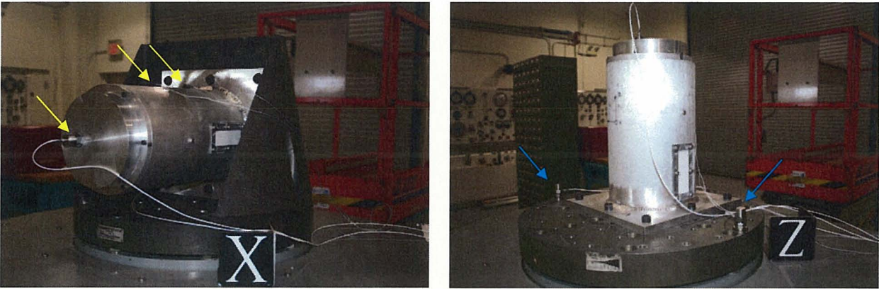
Figure 2. Lateral (X,Y) vibration test fixture with yellow arrows pointing to response accelerometers (left photo) and vertical (Z) vibration test fixture with blue arrows pointing to control accelerometers (right).
