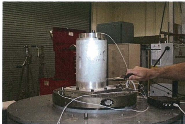
Figure 7 Modal Testing using rubber tipped hammer in Z axis (Response accelerometers opposite).
