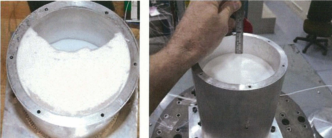
Figure 4 HD Perlite exhibited compaction in the range of 13-17% after X-axis vibration (left) and Z-axis vibration (right). Photographs of typical results.
