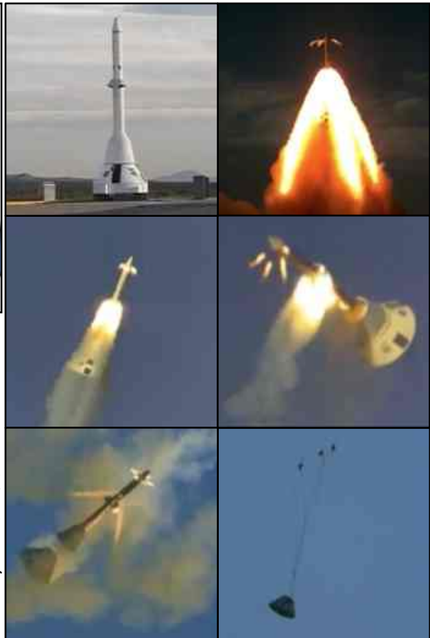
Figure 3. Phases of Orion launch abort flight taken from PA-1 videos (Pad Abort test). From upper left: pre-ignition, boost phase, coast phase, turn around maneuver, tower jettison, and parachute deployment. Note that the PA-1 vehicle was an older configuration with a different aerodynamic fairing shape.
