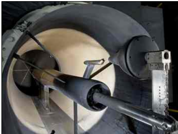
Figure 13. Abort Motor plume CFD validation test in the HFJER at NASA Glenn Research Center. 23
