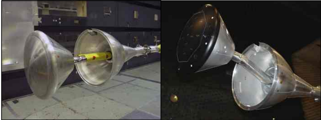
Figure 12. 6%-scale Jettison Motor jet interaction test model in the 14x22-Foot Wind Tunnel at NASA Langley Research Center (left) and 7%-scale model in the AEDC 16T wind tunnel (right).
