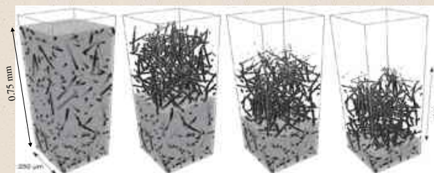
Microscopic scale simulation of the ablation of fibrous materials. J. Lachaud, N. N. Mansour. 48th AIAA Aerospace Sciences Meeting, 4-7 January 2010, Orlando, Florida - Paper 2010-984.
