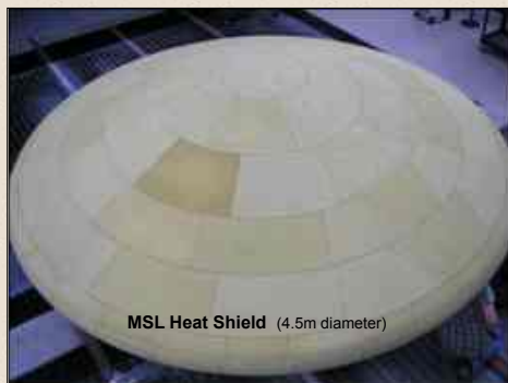
SOA rigid ablators require many tiles to cover large heat shields and require gap fillers
