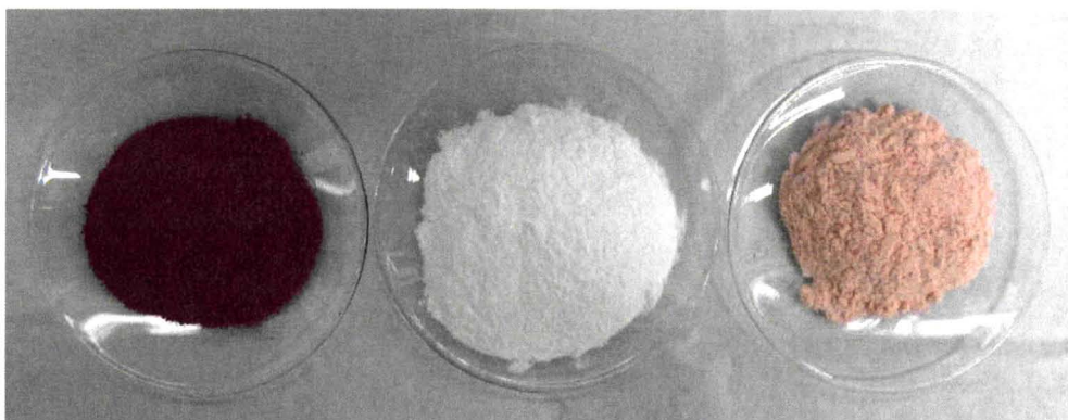
Figure 12. Oil-core microcapsules in free flowing powder form. The core contents of these microcapsules are rhodamine B (on the left), phph (in the middle), and a universal pH indicator (on the right).
