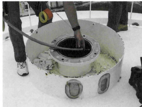
FIGURE 4. Boroscope Being Inserted Into the Annular Relief Opening
