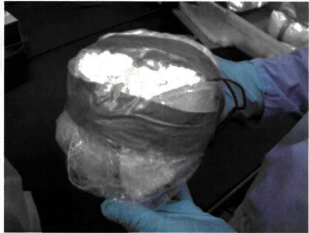
Photo 6. A Maximum Adsorption Garment (MAG, EVA diaper) 'football' from the Shuttle Volume F trash.
