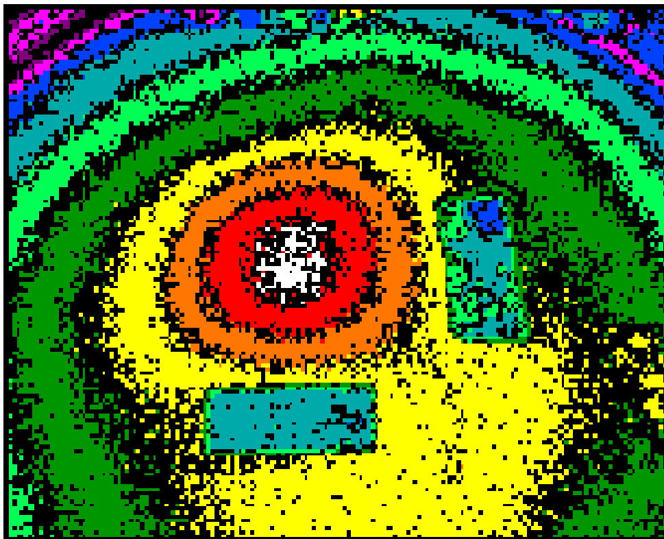
IR Thermographic Image - 35 ft-lbf impact on 10.25 in. dia spherical COPV
