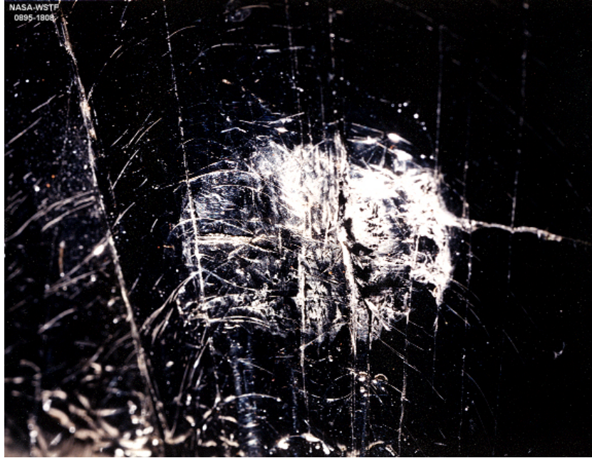
Large Sphere, Unpressurized, 100 ft-lb Impact, 0.5 in. Tup
