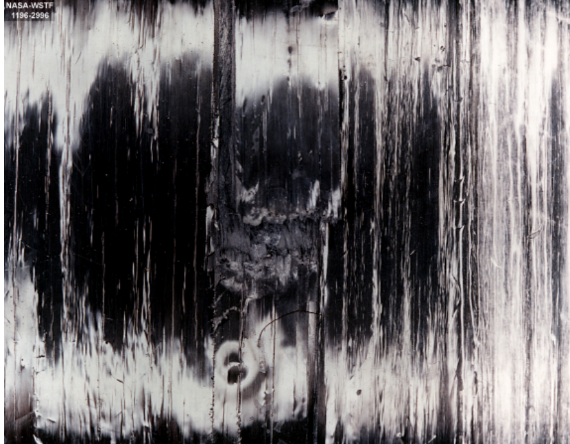
Large Cylinder, 4500 Hydraulic, 35 ft-lb Impact, 0.5 in. Tup, Direct Lighting
