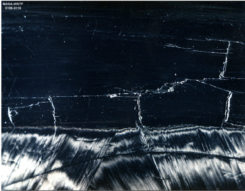
Small cylinder, manufacturing defect, nonelastic end crack
