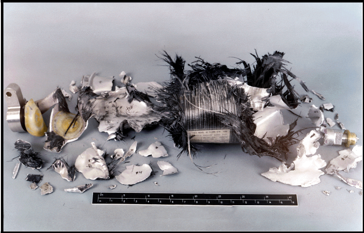
Pneumatic BUI Vessel Posttest
