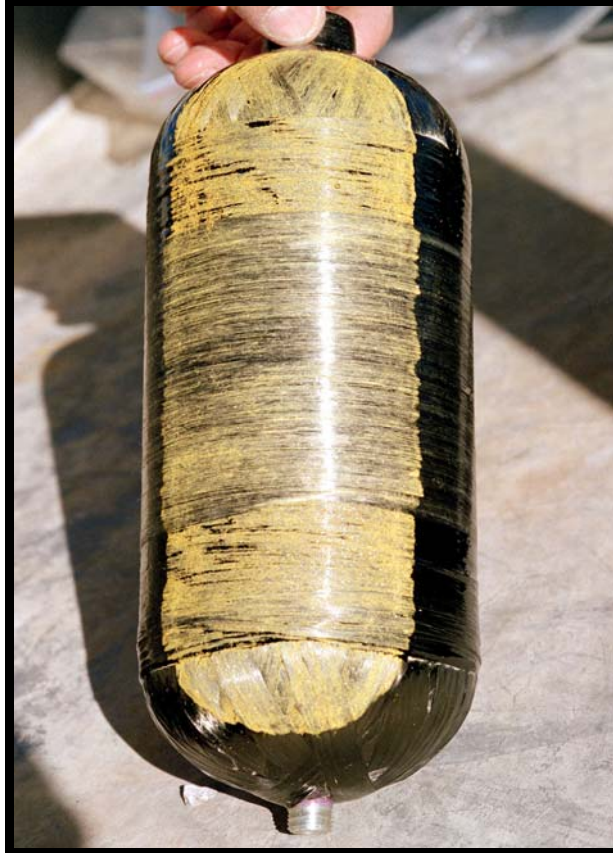
SCI Subscale Vessel after N 2 O 4 Exposure
