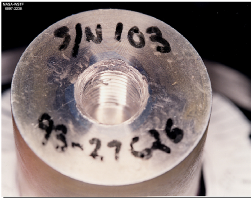
Inlet thread damage
