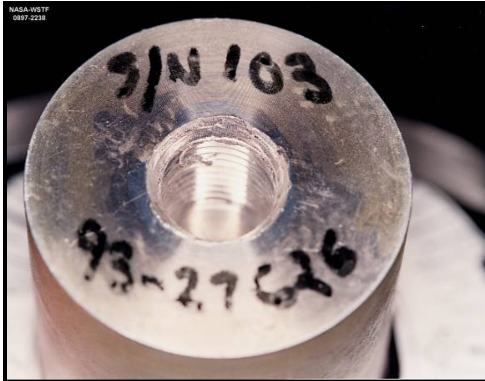
Inlet Thread Damage
