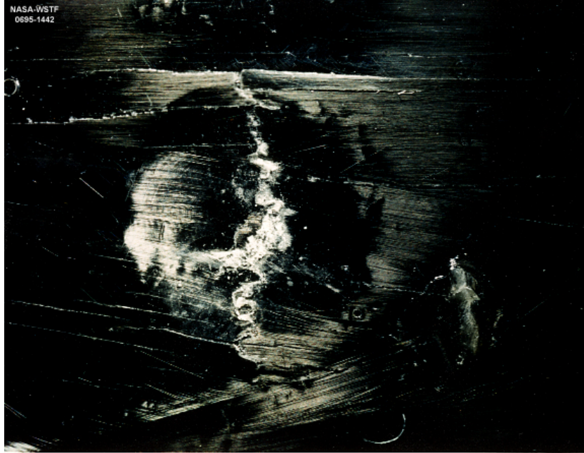
Small Sphere, 6000 psi Hydraulic, 35 ft-lb Impact
