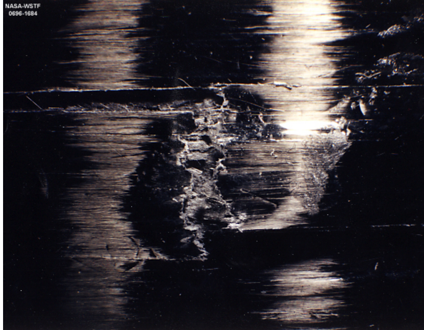
Small Cylinder, 6300 psi Pneumatic, 15 ft-lb Impact, 0.5 in. Tup
