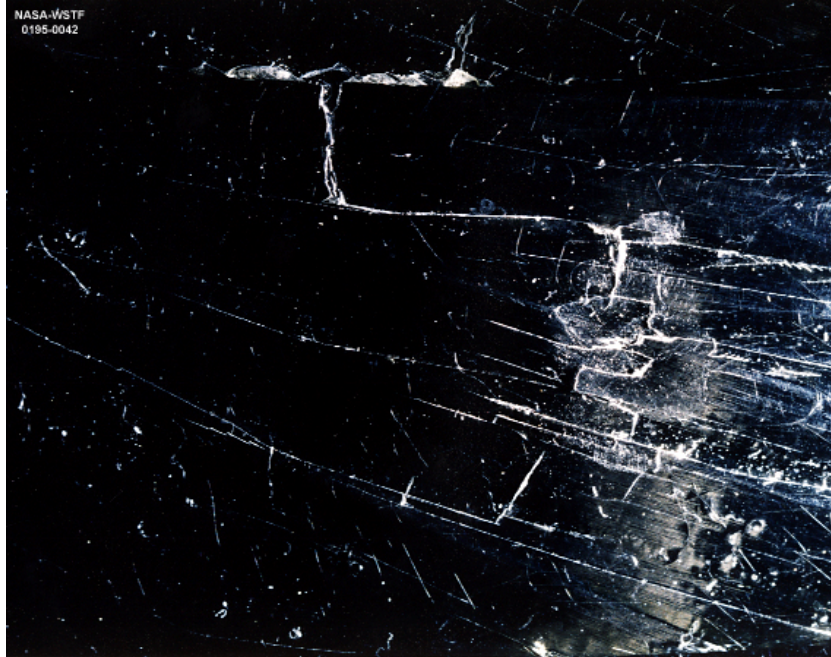
Small Sphere, Unpressurized, 35 ft-lb Impact, 0.5 in. Tup
