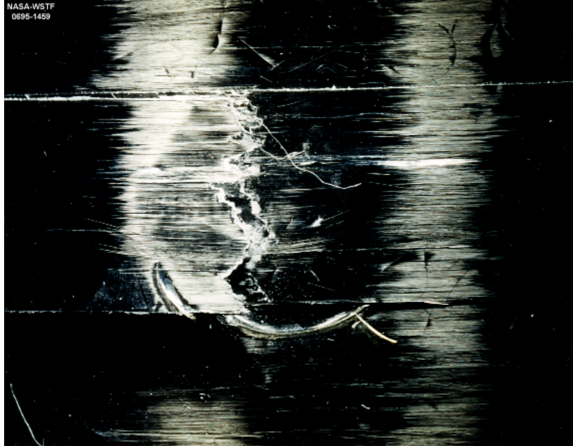
Large Cylinder, Unpressurized, 65 ft-lb Impact, 0.5 in. Tup
