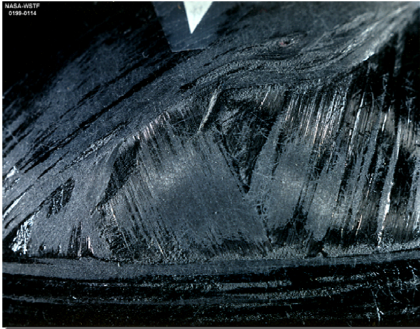
4.6 x 10 in. cylinder, significant abrasion
