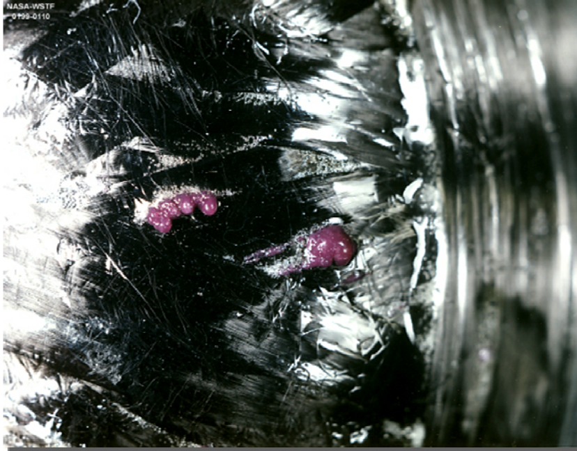
4 x 9 in. cylinder, excess bonding agent
