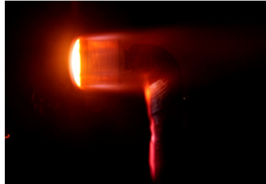
Figure 5. TPS sample with internal WLSS being heated in the AHF arc.
