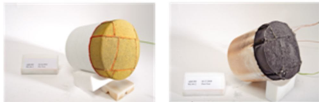
Figure 2. TPS sample pre-test (left) and post test (right).
