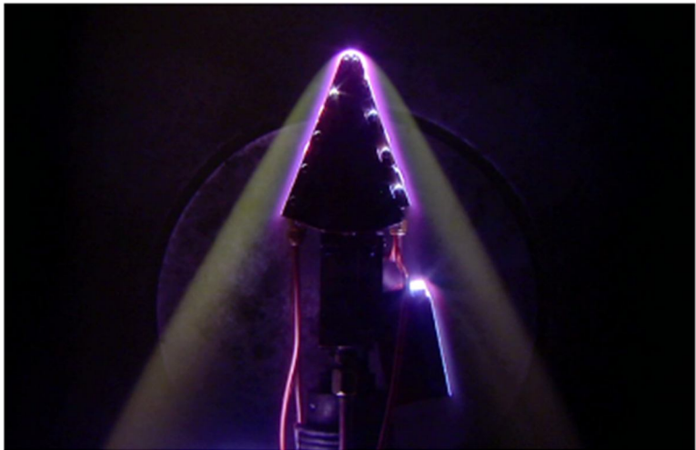
Figure 12. WLSS in the test wedge inserted into the flow from the IHF arc jet.
