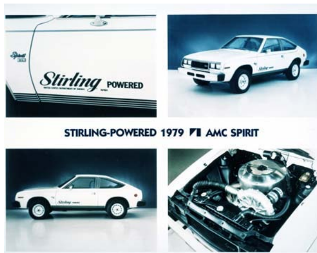
Figure 5.—A Stirling powered vehicle researched by NASA in the 1970's.
