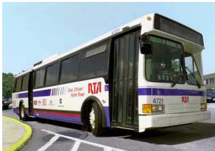
Figure 8.—The NASA Hybrid Electric Transit Bus (HETB).
