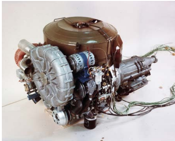
Figure 6.—A Stirling engine researched by NASA in the 1970's.
