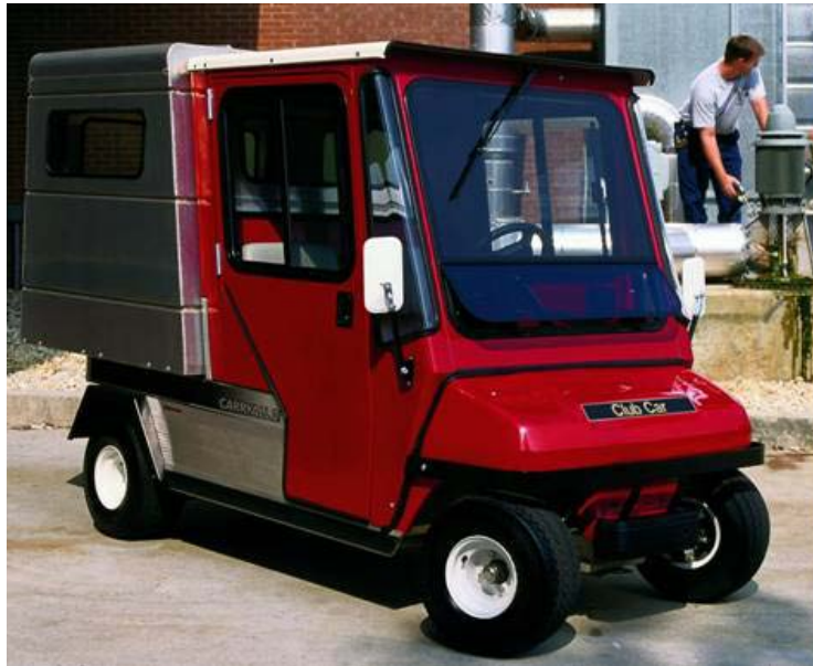
Figure 10.—A fuel cell powered utility vehicle equipped with ultracapacitors.
