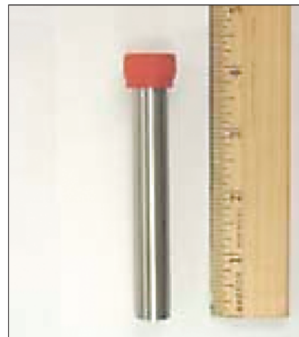
A TSEV is a test-tube-like stainless-steel vessel that can be purged with a gas and immersed in a hot oil bath.
