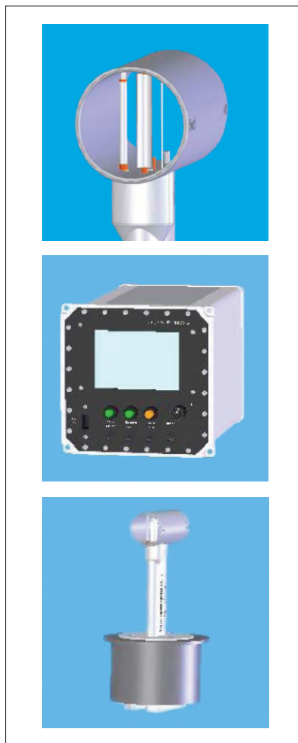
The Sensor Head (top) contains three hot-wire sensors oriented perpendicularly to the axis of the tube (across the flow) and one parallel to the axis of the tube (along the flow). The general views of the cockpit display and the sensor are shown, respectively, in the middle and bottom images.
