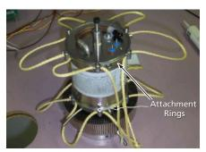
ASSEMBLY STAGE 1: CORDS LACED THROUGH HOLES IN ATTACHMENT RINGS
