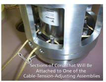
ASSEMBLY STAGE 2: CRYOCOOLER IN CAGE, CORDS LACED THROUGH HOLES IN CAGE
