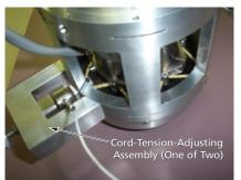
ASSEMBLY STAGE 3: CRYOCOOLER SUSPENDED BY TENSIONED CORDS
