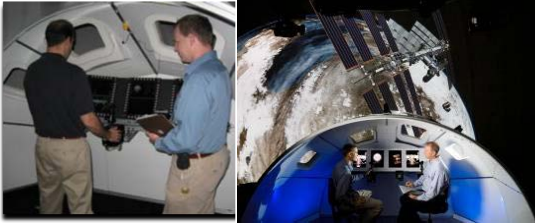
Figure 3. The ROC facility. The left shows the actual setup (illuminated by the camera flash) and the right shows the type of out-the-window scene generation capability that was used.
