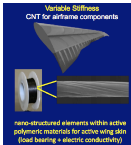
Figure 5. Carbon-nanotube material applications for airframe components.
