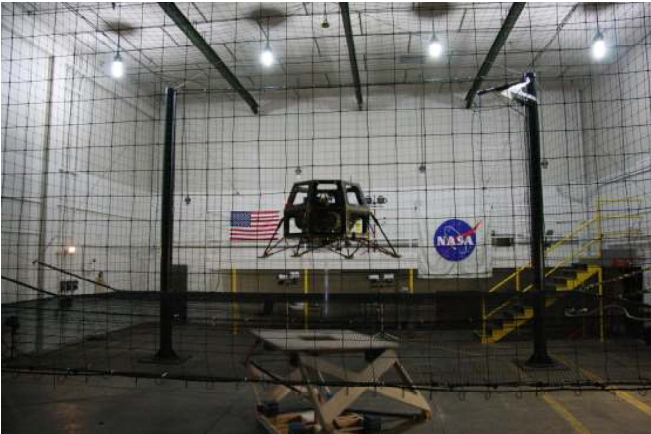
Figure 20: Image of free flight hover test shortly after liftoff. The main engine gas stream (and associated mach diamonds) are visible.
