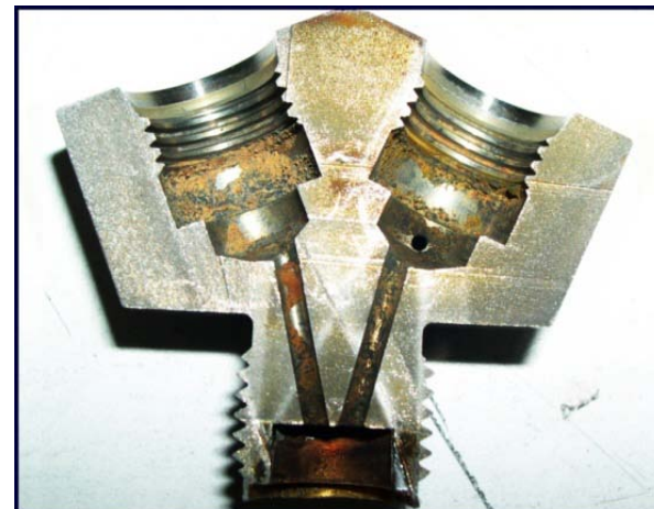
Posttest, Sectioned Stainless Steel V-PCA
