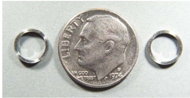
Figure 5. Sealing Rings Shown Alongside a U.S. Dime.
