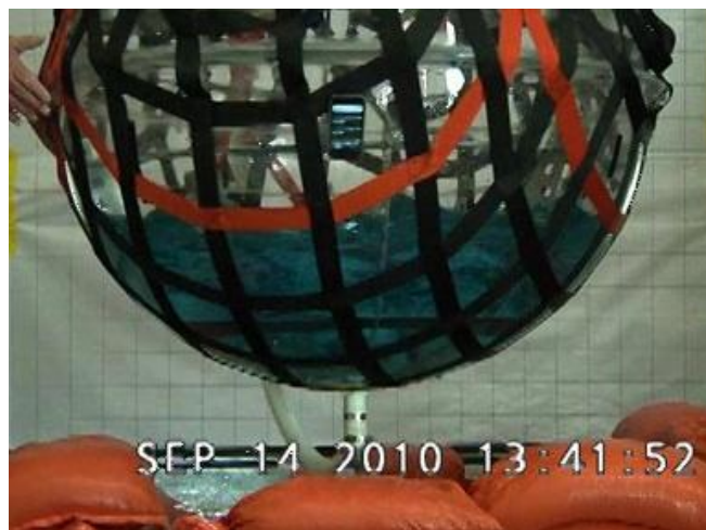
fig-11, Baffles damping slosh at 20 % full
