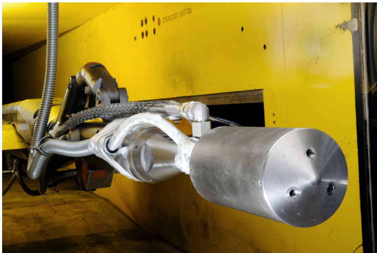
Figure 1: Mounting apparatus and the 5''-diameter model with 3 nozzles as installed in test section 2 of the NASA Langley Unitary Plan Wind Tunnel. 24
