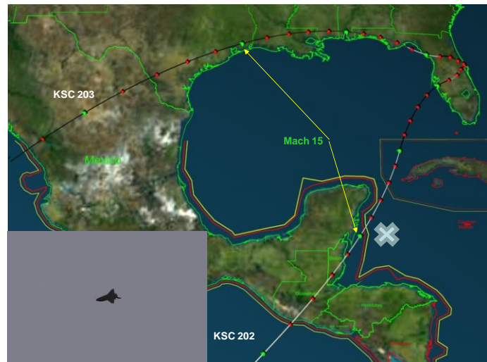
Figure 4. Graphical output from the ViDI Entrysim3D toolset includes trajectories with integer Mach numbers indicated by dots. Global display includes political borders and foreign airspace boundaries. The inset image is a simulated camera view of the Orbiter as it passes the airborne imaging asset indicated by the large “X” in the image.
