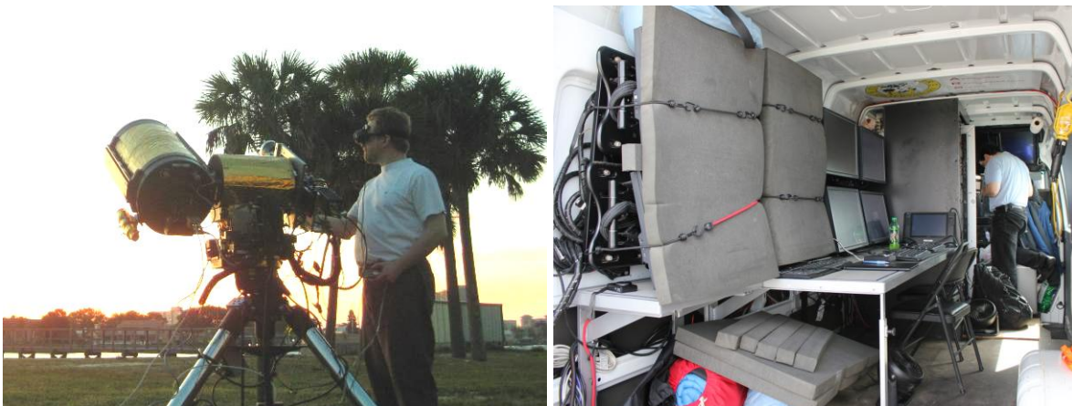
Figure 14. MARS Mobile telescope system. On left is the telescope and camera on mount. Note the operator’s video display goggles, which provide a clear view of the video feed under all lighting conditions. On the right is the mobile support van with controlling and processing computers. Images are from the STS-133 deployment.
