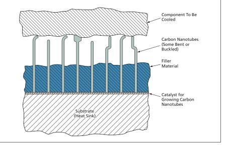
**Carbon Nanotubes Bend and Buckle** to accommodate roughness of the surface of the component to be cooled. The high longitudinal thermal conductivity of carbon nanotubes is exploited to conduct heat into the heat sink.
