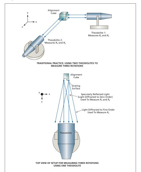
Two Theodolites are needed to measure rotations about all three Cartesian axes in traditional practice using a purely specular alignment cube. Applying a diffraction grating to one face of an alignment cube makes it possible to measure all three rotations using a single theodolite.
