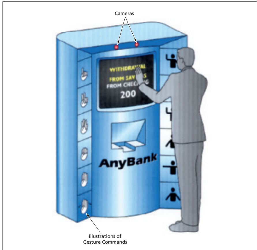
A User Would Control an Automated Teller Machine through gestures. Panels on the sides of the machine would depict static and dynamic hand and arm signals recognized by the system.
