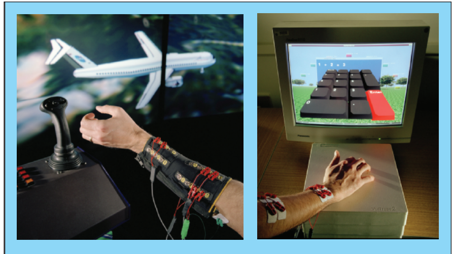
Electrodes on a Subject's Forearm were used to acquire EMG signals in experiments on synthesizing joystick attitude controls for simulated airplane flight and synthesizing typing on a numerical keypad.
