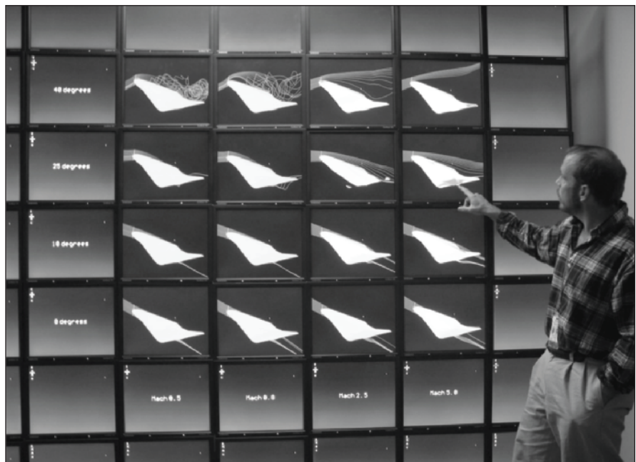
Figure 2. Each of 16 Images displayed on a hyperwall represents results of a computational simulation of airflow about an aerospacecraft (specifically, a proposed reusable launch vehicle) at one of 16 different combinations of Mach numbers and angles of attack.
