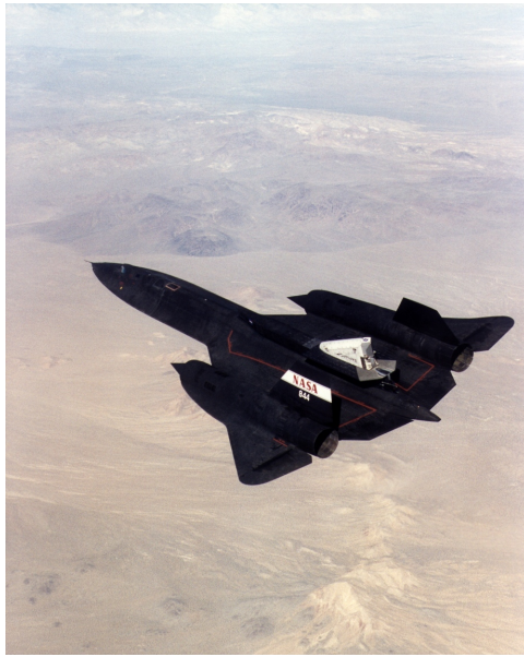
Figure 1. The Lockheed SR-71 Blackbird in flight with the Linear Aerospike SR-71 Experiment (LASRE) attached.
