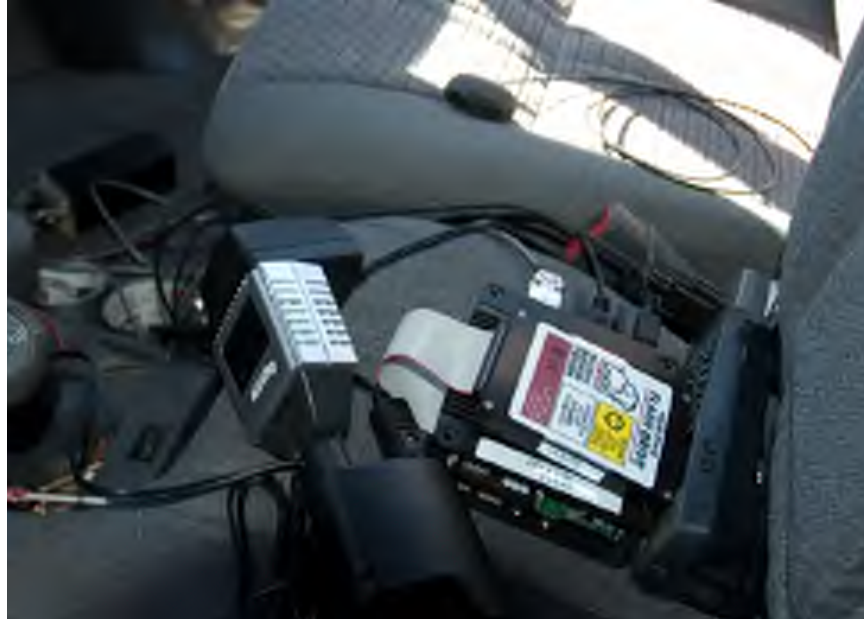
Figure 14. REVEAL on eBox-2300 - field test setup
