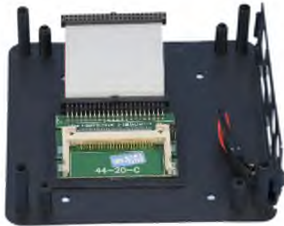
Figure 12. Attachment of PATA-CF adapter to eBox baseplate
