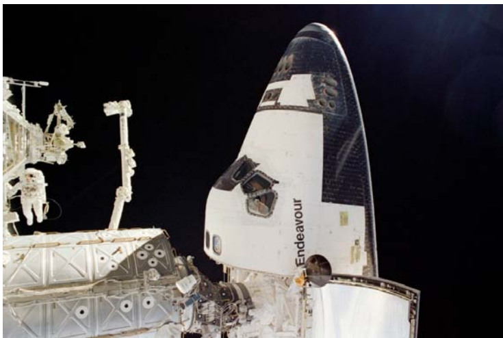
Figure 67 – Space Shuttle Orbiter attached to PMA-2 at the forward axial port of the U.S. “Destiny” laboratory.
