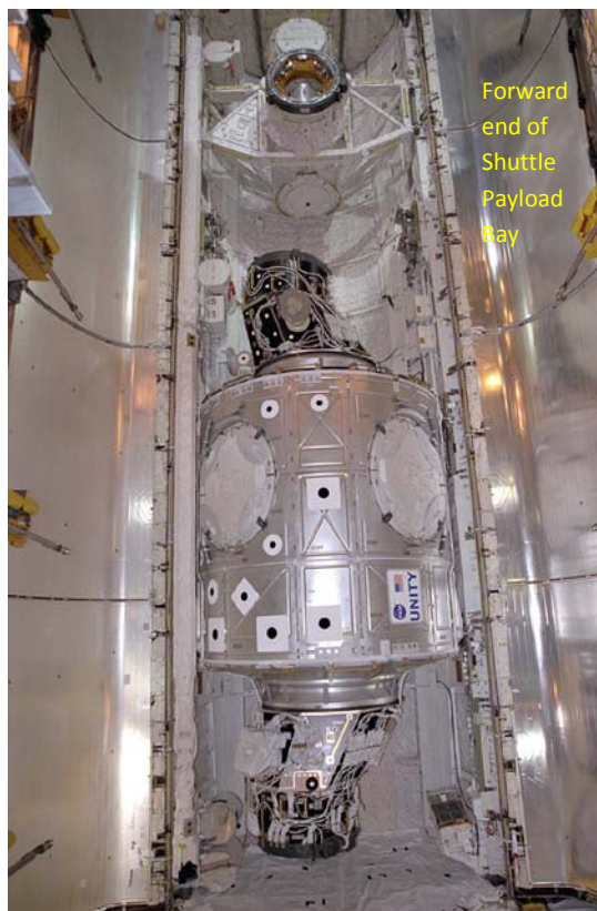
Figure 11 – “Unity” Node in the Orbiter Payload Bay. PMA-2 is forward in the bay, PMA-1 is aft in the bay.
