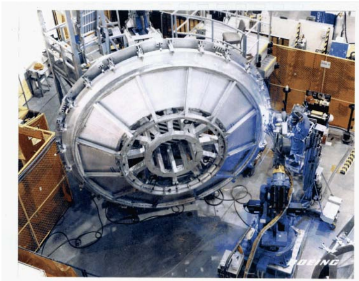
Figures 5 –Overview of welding fixture at The Boeing Company, Huntsville, AL.
