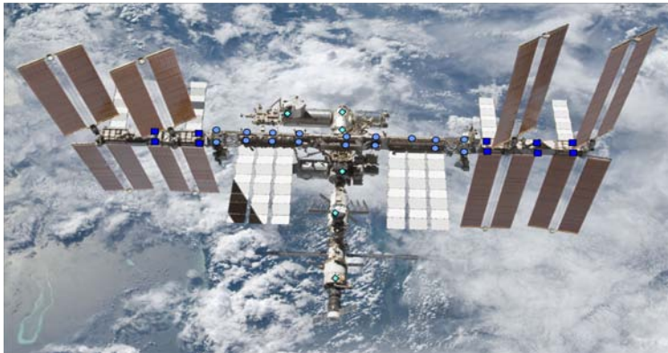
◆ IWIS - Internal Wireless Instrumentation System ● SDMS – Structural Dynamic Measurement System ■ EWIS – External Wireless Instrumentation System
