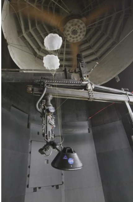
Figure 2. Orion Crew Module with drogue parachutes in Langley 20-Foot Vertical Spin Tunnel.
