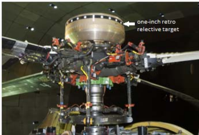
Figure 8. Instrumentation hat with one-inch diameter retro-reflective targets installed.
