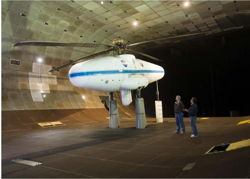
Figure 1. UH-60A Airloads rotor system installed on LRTA in the NFAC 40- by 80-foot test section.
