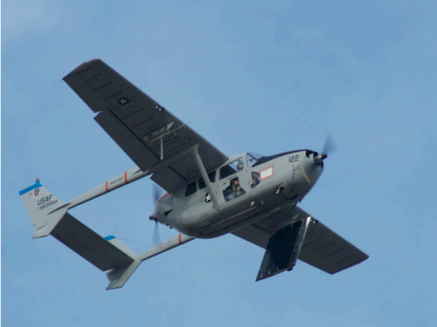
Fig. 18. Model mounting and initial pitot-static location on the Cessna O-2 flight platform.
