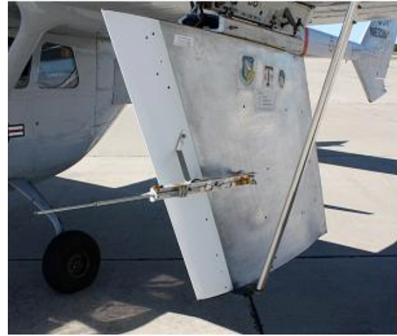
Fig. 19. Placement of the 5-hole probe on the model.
