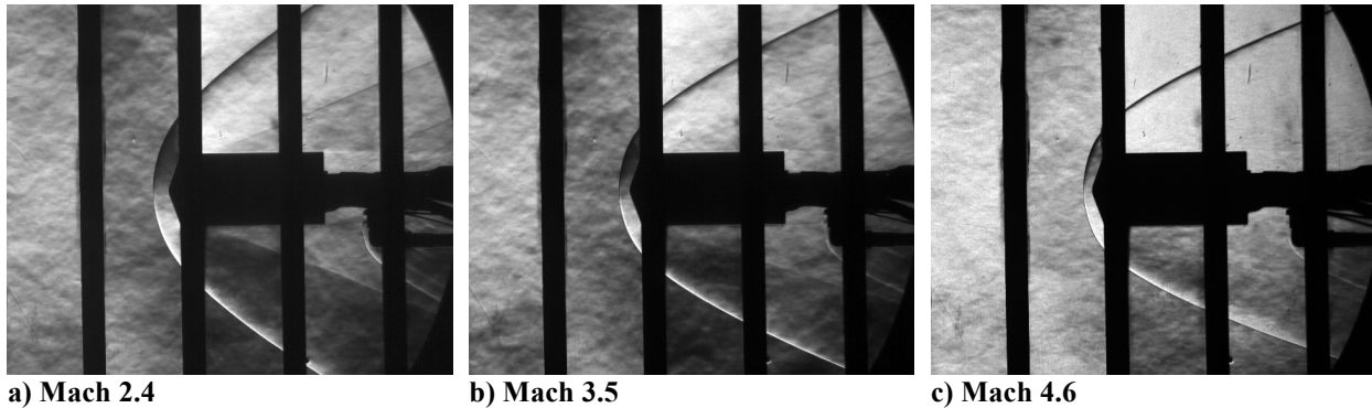
Figure 12. Effect of Mach number for the baseline configuration at \alpha = 0 -deg
