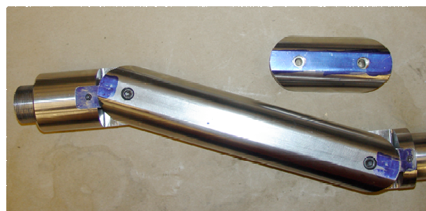
Figure 10. Photograph of Test 24-AA Articulated Sting with Short and Long Links.
