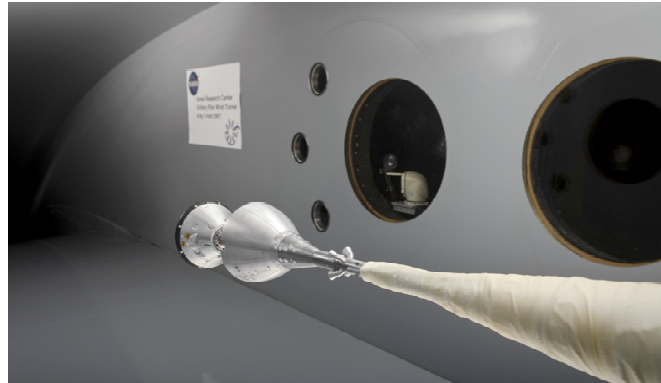
Figure 15. Test 25-AA Model in NASA Ames 9x7-Foot SWT.
