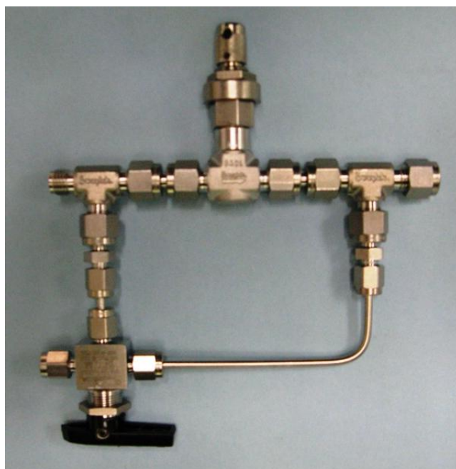
Figure 2. OGA Single Cell Microbial Challenge Sample Valve.
