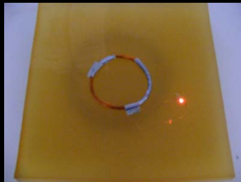
Coil powering an LED
