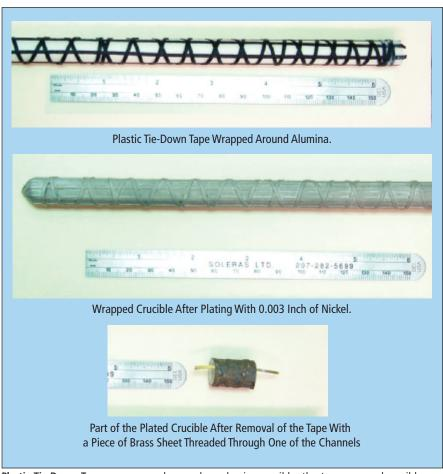
Plastic Tie-Down Tape was wrapped around an alumina crucible, the tape-wrapped crucible was electroplated with nickel, then the tape was burned out, leaving nickel-walled passages covering the crucible.
