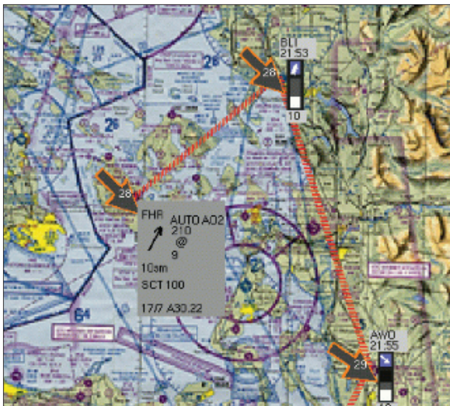
Current Weather and Winds Aloft are shown alongside a pilot-selected route. Wind velocity at the pilot-selected altitude is depicted graphically with black arrows. The current weather is shown using symbolic and textual representations.
