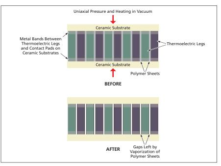
A **Single Thermoelectric Module** containing a small number of legs is shown here for simplicity to facilitate understanding of the process described in the text. In an economically practical version of the process, multiple modules would be stacked in a more-complex, checkerboardlike arrangement during bonding and vaporization of the polymer sheets.
