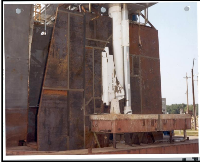
Figure 5-3. Acoustic Model Test Facility - 6.4% Shuttle Model
