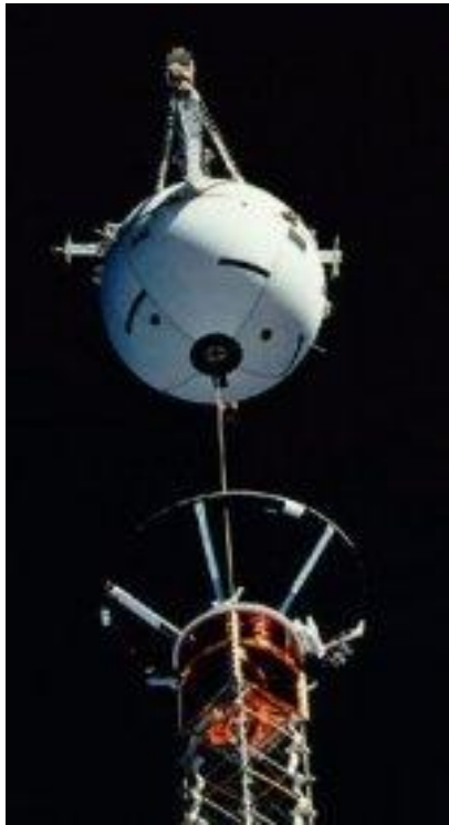
Figure 24-1. Tethered Satellite and Level Wind Mechanism
