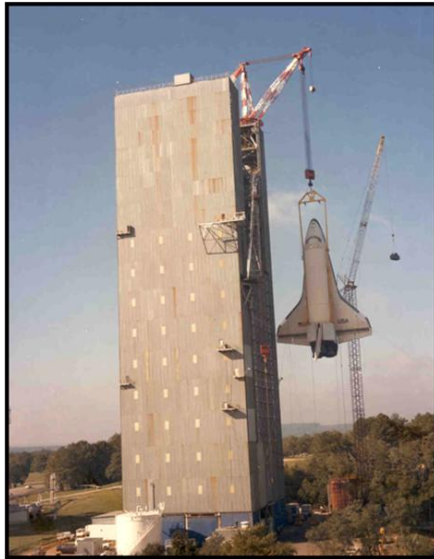
Figure 19-1. Shuttle Orbiter Being Installed Into Dynamic Test Stand
