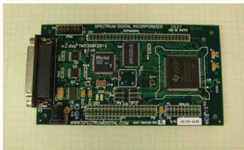
Figure 2. The SAFE prototype—DSP hardware version
