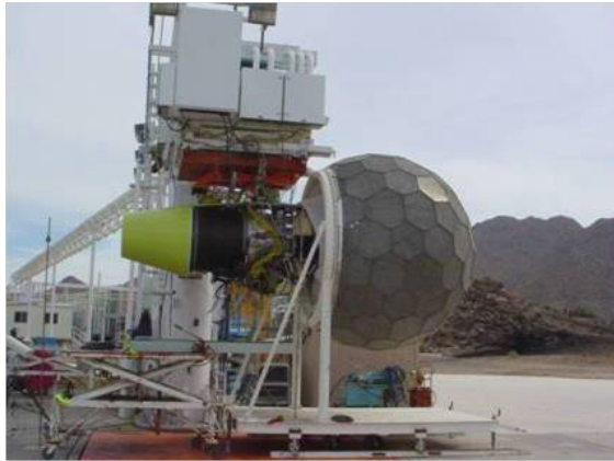
(a) Tech977 turbofan engine mounted on test rig with ICD
