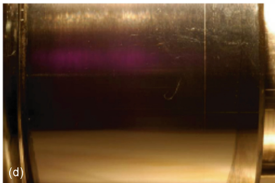
Figure 6.—Wave bearing rotor with SiDLC coating at decreasing oil supply pressure (OSP) (from [10]). (a) 1st hour at 0.07 MPa. (b) 2nd hour at 0.035 MPa. (c) 3rd hour at 0.01 MPa. (d) 4th hour at 0 MPa.
