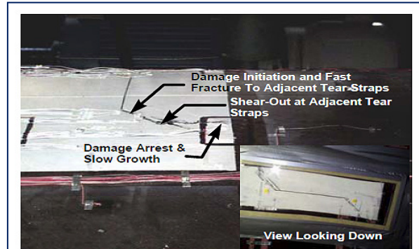
Figure 6.3-16: Photograph of Failed Fuselage Panel
