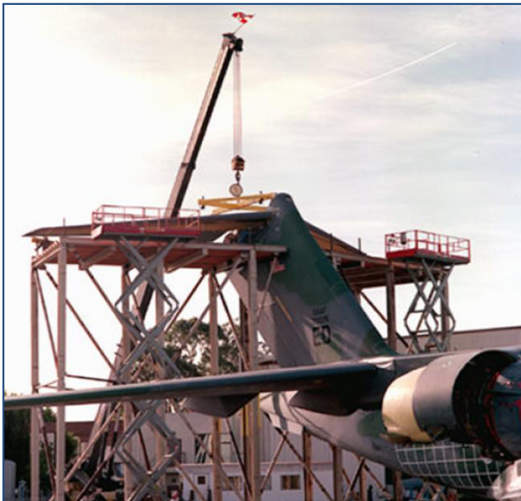
Figure 2.4-2: C-17 Horizontal Tail Redesigned Using Composite Materials
