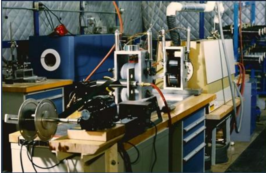
Figure 12.8-3: Photograph of the Ribbonizing Line Installed at LaRC in Building 1293C
