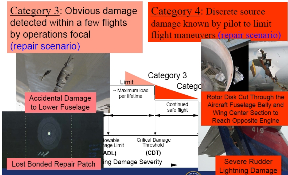
Figure 15.1-3: FAA Categories of Damage for Composite Aircraft Structure and Selected Examples of Damage on Actual Aircraft
