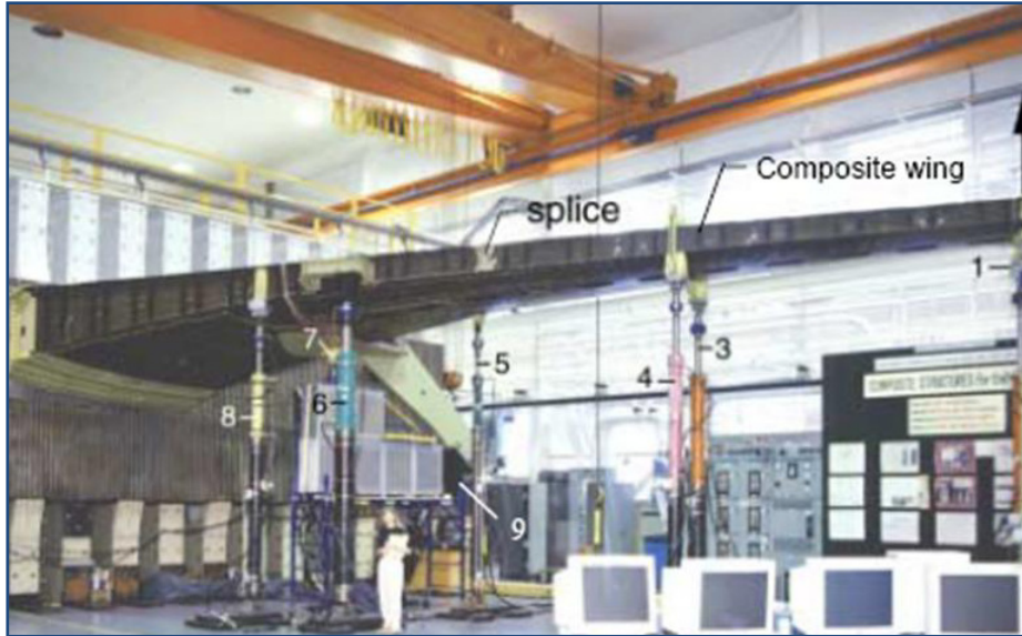
Figure 4.5-16: Semi-span Wing Prior to Testing at NASA Langley
