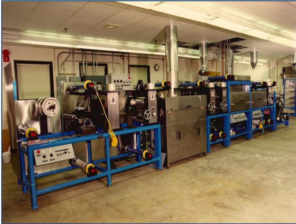
Figure 12.4-1: Modular Horizontal, Automated Prepregger Installed at LaRC
