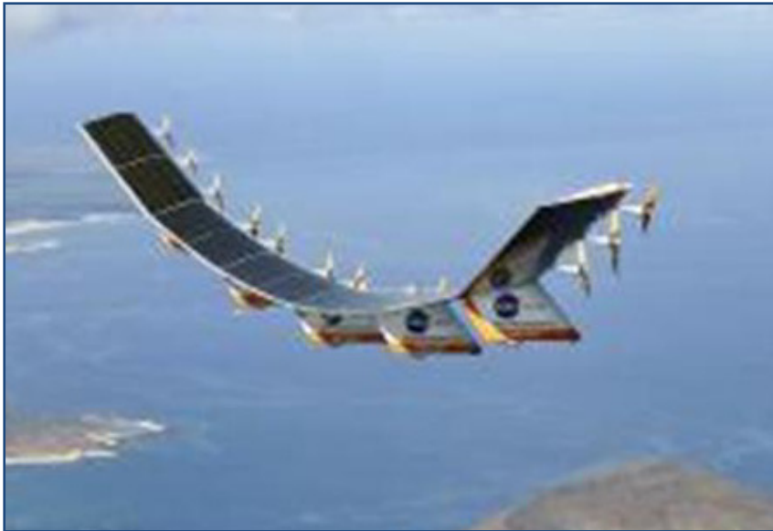
Figure 2.6-1: The Solar-electric Helios Prototype Flying Wing is Shown Near the Hawaiian Islands of Niihau and Lehua During its First Test Flight on Solar Power
