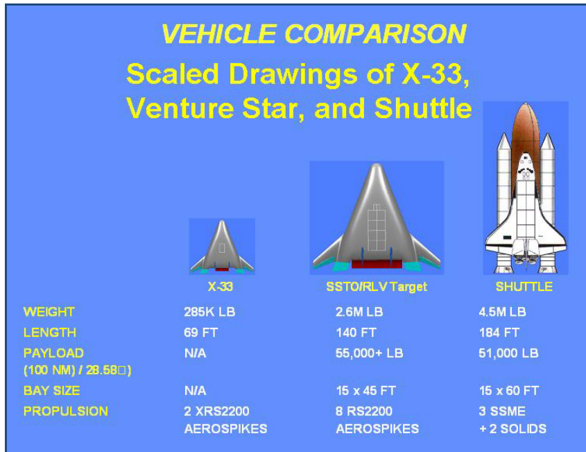
Figure 9.3-4: Scaled Drawings of X-33, Venture Star, and Shuttle for Comparison
