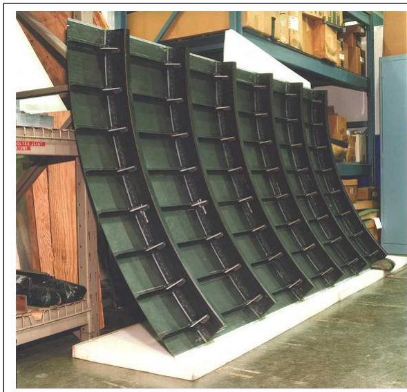
Figure 6.3-1: High-Temperature IM-7/PETI-5 Skin Stringer Panel (6'x10')
