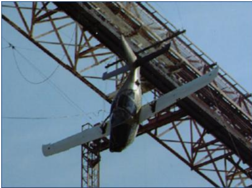
Figure 7.2-3: AGATE Composite Airframe Impact Test
