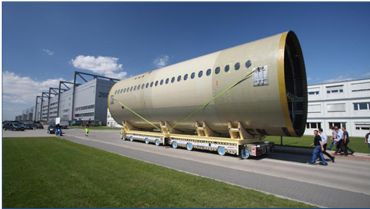
Figure 2.1-5: Test Fuselage Section for the Airbus (Toulouse, France) A350 XWB Aircraft
