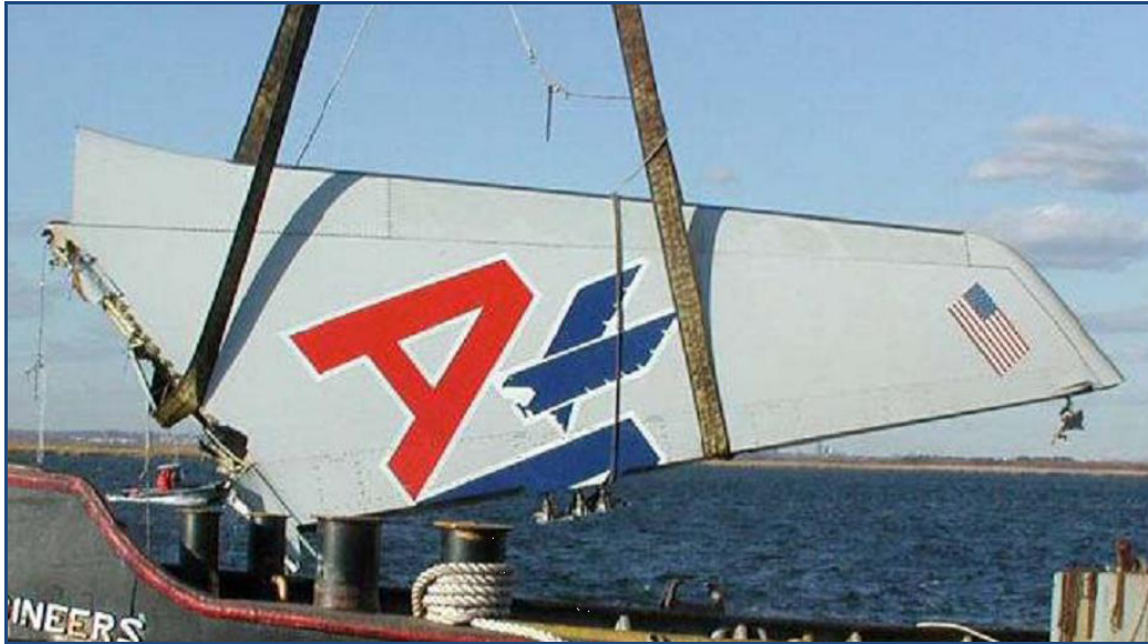
Airbus 300-600R Vertical Tail Plane (VTP) Recovered American Airlines Flight 587
