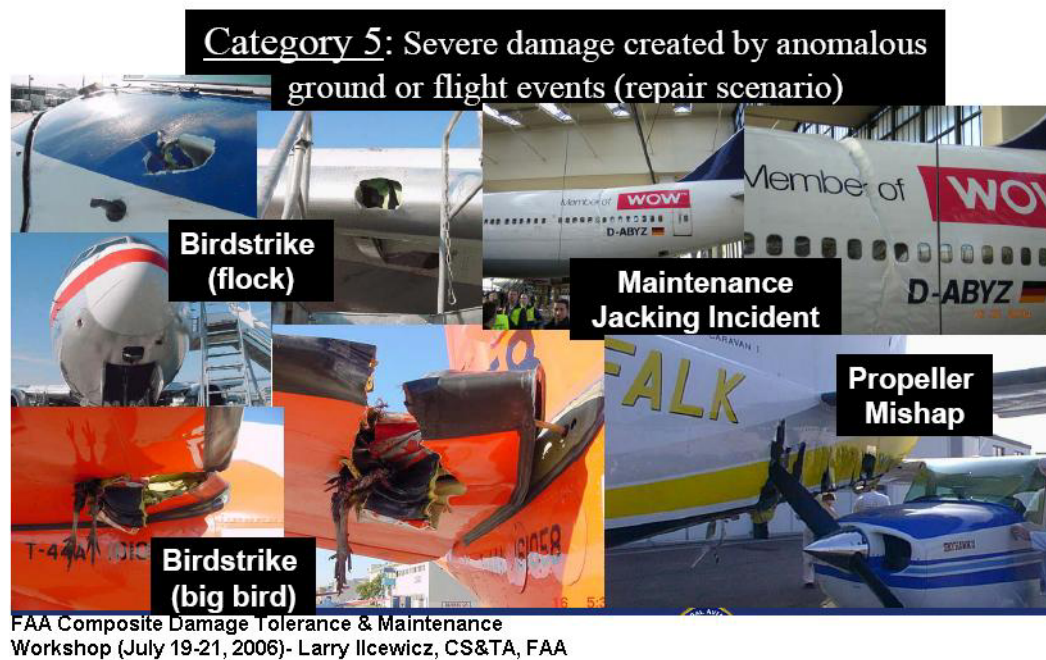
Figure 15.1-4: Examples of Category 5 Damage to Aircraft
