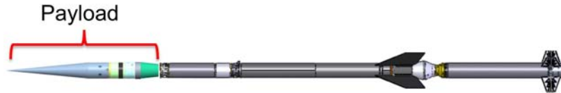
Figure 3.1: Black Brant X with IRVE-4 Payload
